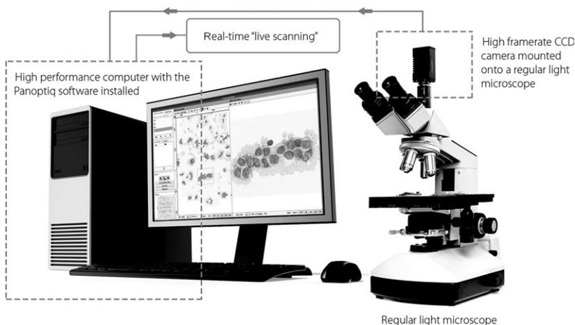
**Figure 1.** Illustration of the Panoptiq systems Setup - Image is captured through the high framerate camera as the user views the peripheral blood film on the microscope. Subsequently, the image output is processed through the high performance computer using the Panoptiq software which facilitates the real-time "live scanning" of the captured image into a panoramic image.
